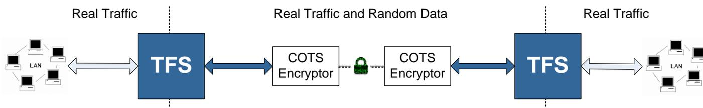
The Traffic Flow Security (TFS) device masks the transmission of information in order to prevent interception and/or analysis of traffic patterns and characteristics. TFS is of particular importance in military applications where the activity pattern can indicate the possibility of an action being planned or executed. By intercepting and analyzing the flow of information, even encrypted information, an enemy would be able to determine the status of an operation.
