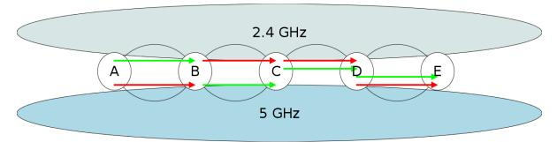
With network-wide multi interface optimization a multi-interface node can act as a routing splitting point. In the example below node B will route the packets via C if they are coming from F (green path) and route the packets via G if they are coming from A (red path) for the destination E. This is different from the previous implementation since packets are routed based on the interface received rather than via the same path.
