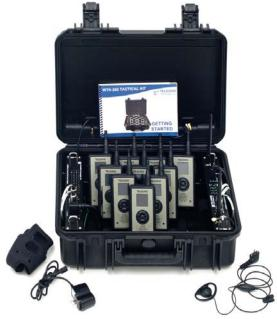
WZRDnet is a wireless ad-hoc mesh network that provides voice and data communications without existing infrastructure (i.e. no cell towers or satellites required). WZRDnet Kits contain, in a single man-transportable case, all the equipment needed to form a complete stand-alone voice, text and data mesh network as well as provide Wide Area Network access.
